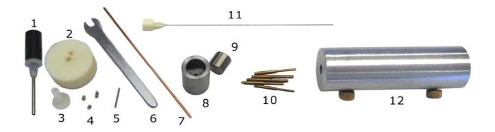
1,2,3, - cutting device for rubber sealling; 4 – rubber seallings; 5 -force out pivot; 6 – key; 7 – push out pivot; 8,9 – sample preparation device; 10 – pistons; 11 – rubber sealling extractor; 12 – cell holder.
