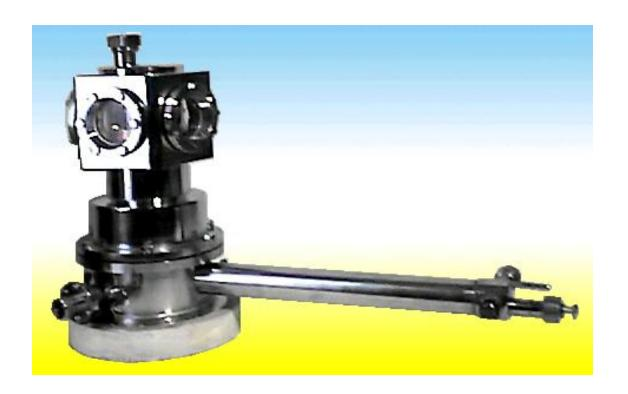
Cryostats of "CTR" series are designed for transmission and reflection coefficient measurements of different samples in temperature range from He to room temperatures.
