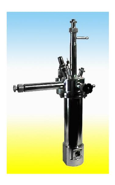
Small size cryostats of "CT" series are designed for transmission coefficients measurements of different optical samples of temperature in range from helium to room. The "CT" series is presented by three cryostats for samples with diameter up to 25, 50, 75 mm.
