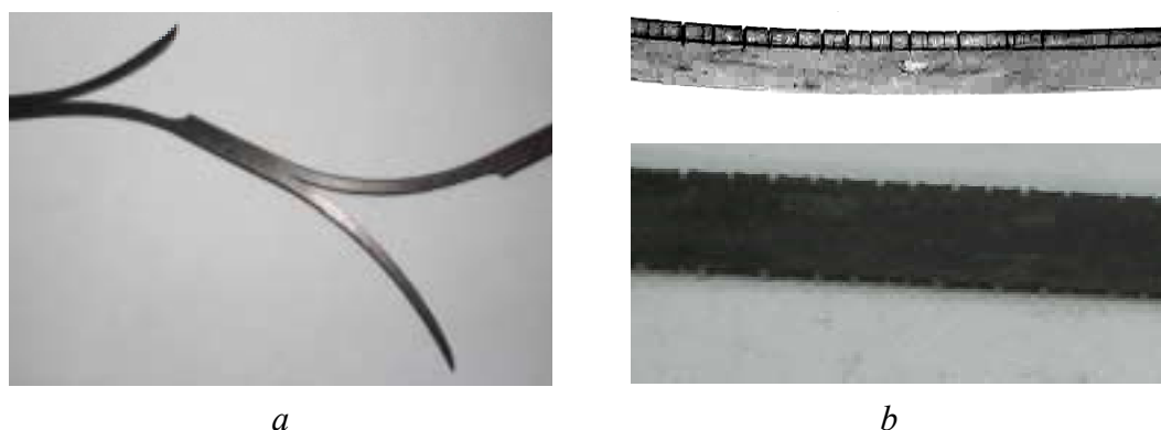
Fig. 2. Sample view after cold rolling without (a) and with (b) current
