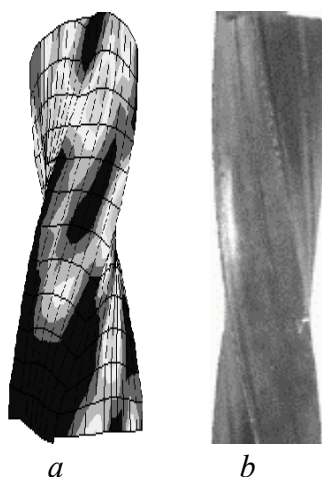
Fig. 4. Schematic (simulation results) ( a ) and photo (experimental results [9]) ( b ) of twist sample after one-pass deformation
